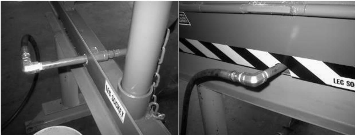
7. Check the routing of the temporary hydraulic lines to assure that the hose is clear of legs, base frame, and platform when lift is in the lowered position.
