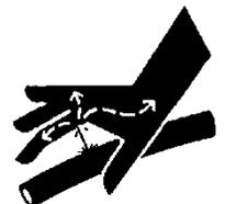
**Hydraulic hoses can fail from age, damage and exposure. Do not search for hydraulic leaks without body and face protection. A tiny, almost invisible leak can penetrate the skin, requiring immediate medical attention.**
