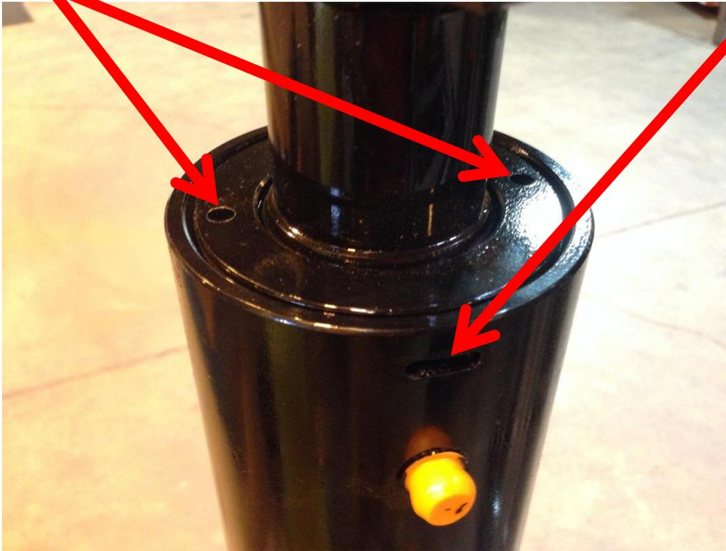
2. Place a small screwdriver under retainer and turn retainer to remove.
