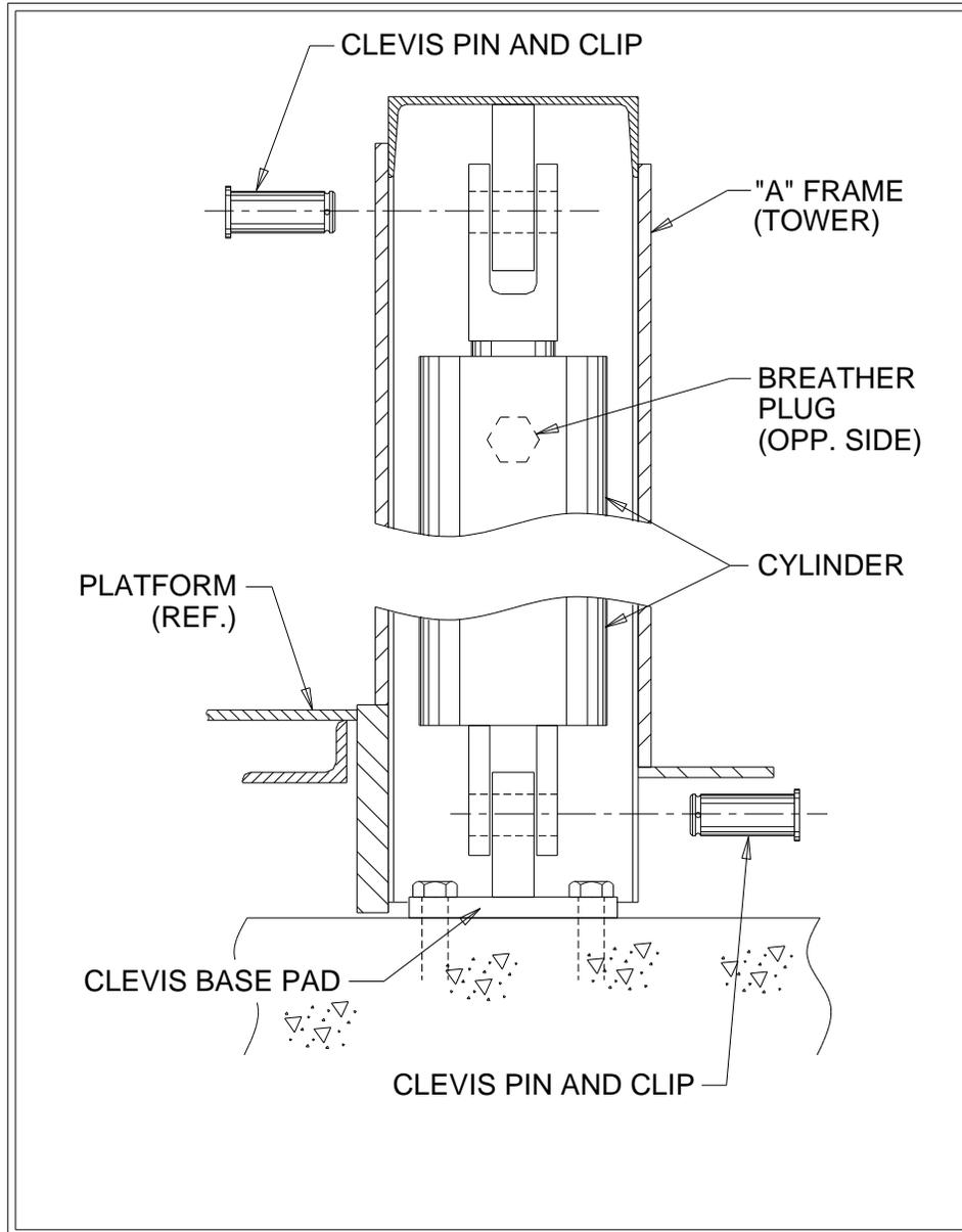
**Figure 9 Cylinder & Tower Installation**
