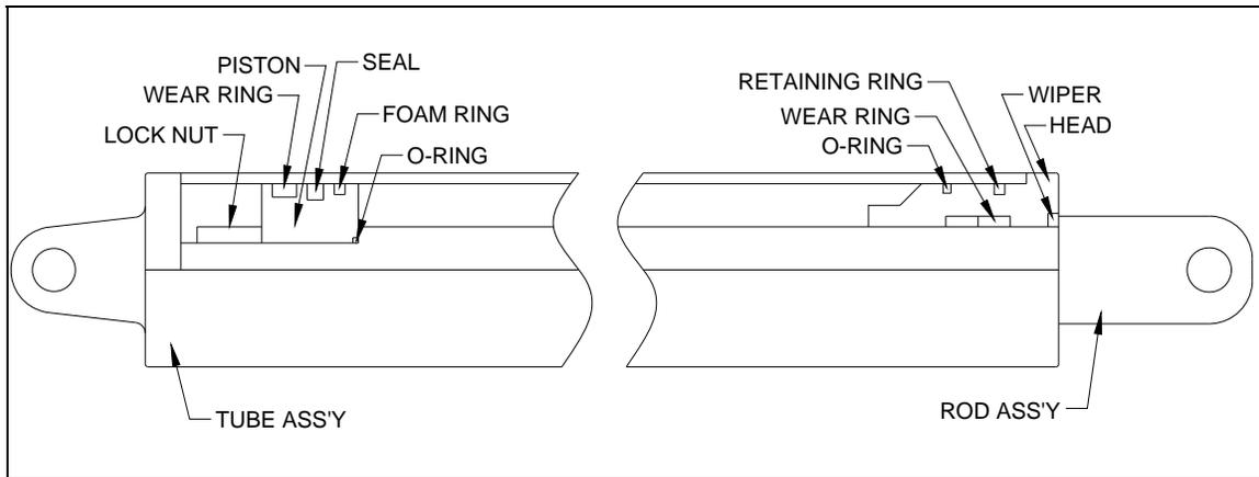
**Figure 12 Double Acting Hydraulic Cylinder**
