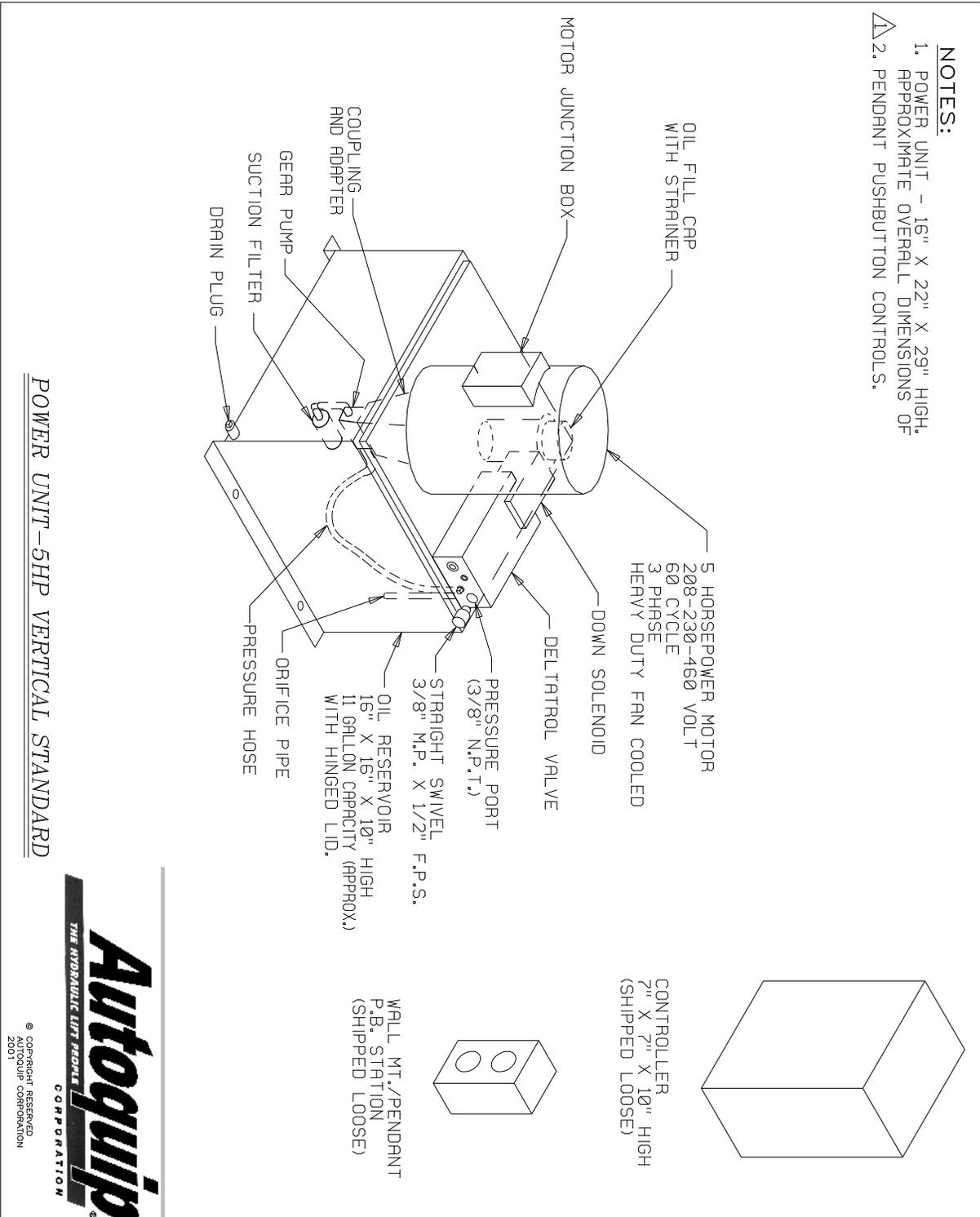
Figure 20 Vertical Power Unit Parts Detail
